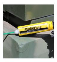
7. Larger repairs (larger than 2") may benefit from adding another layer of repair material. Cut the second piece of fabric so that it overlaps the initial repair by ¼ to ½ inch. Then simply repeat steps 4 to 6. This may be performed immediately, or after the first repair has cured. The repaired area may be spray painted immediately after application, and soil and sod may be replaced.
